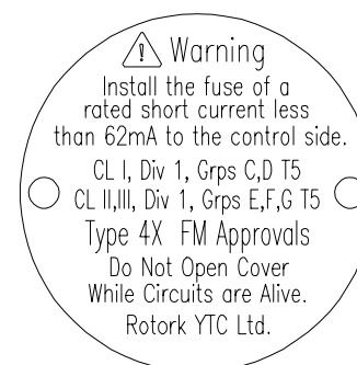
图L-8: YT-1000 CL I, Div 1, Grps C,D T5; CL II, III, Div 1, Grps E,F,G T5; Type 4X (FM)
